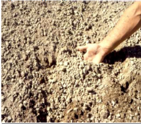
Figure 24: Typical granular embedment
